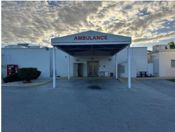
LKMC121a 1/27/2026 Ambulance entry lacking accessible curb ramp East elevation
